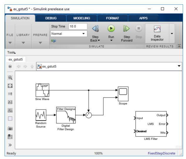
4 Set the LMS Filter block parameters to model the output of the Digital Filter Design block. Open the LMS Filter dialog box by double-clicking the block. Set and apply the block parameters as follows:
