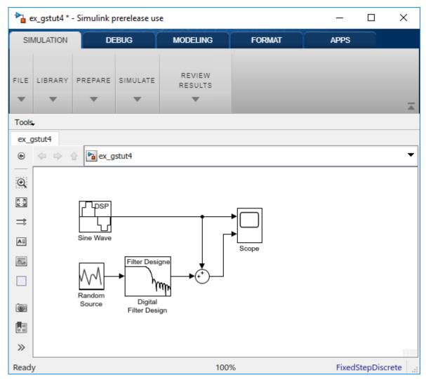
**3** Run your model and view the results in the Scope window. This window shows the original input signal and the signal with low frequency noise added to it.
