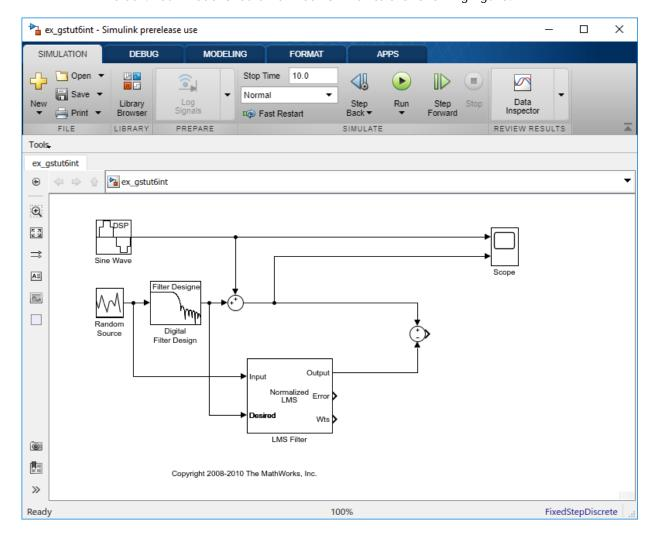
The positive input to the second Sum block is the sum of the input signal and the low frequency noise, s(n) + y. The negative input to the second Sum block is the LMS Filter block's best estimation of the low frequency noise, y'. When you subtract the two signals, you are left with an approximation of the input signal.
